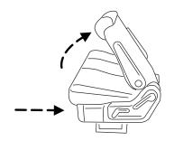
Before returning the seatback to its original position, make sure that cargo or any objects are not trapped underneath the seatback. After returning the seatback to its original position, pull on the seatback to ensure that it has fully latched. An unlatched seat may become dangerous in the event of a sudden stop or collision.
